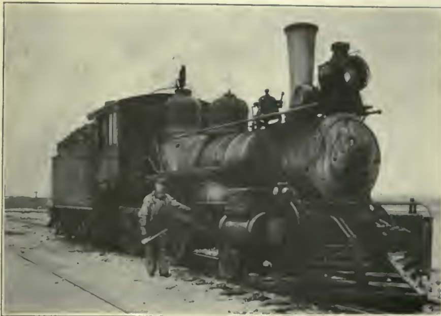
FIG. 382. LOCOMOTIVES. Passenger Locomotive of the American Type. One of the older and lighter of the passenger loco- motives used in Chicago, now engaged in Suburban Service. Wabash Railroad.
